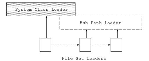
A "base" class loader is used to handle course changes to the classpath including added path. Unless directed by setClassPath() the base loader will only add path and will not cover existing Java user class path. This prevents unnecessary class space changes for the existing classes.
