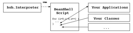
You can use BeanShell to run scripts from the command line or enter statements interactively by starting the bsh.Interpreter class. (See "Quickstart" for instructions on adding BeanShell to your classpath.)
