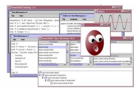
The BeanShell Desktop is a simple GUI environment that provides multiple bsh shell windows (MDI), a simple text editor, and a simple class browser. The desktop is mostly implemented by BeanShell scripts, launched by the desktop() command.
