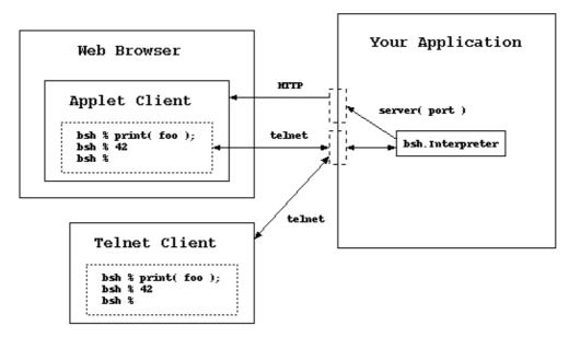
Remote server mode lets you access a BeanShell Interpreter inside of a remote VM. With remote server mode activated you can literally telnet into the running application and type commands at the BeanShell shell prompt. Or, even better, you can use any web browser to bring up a remote GUI console.
